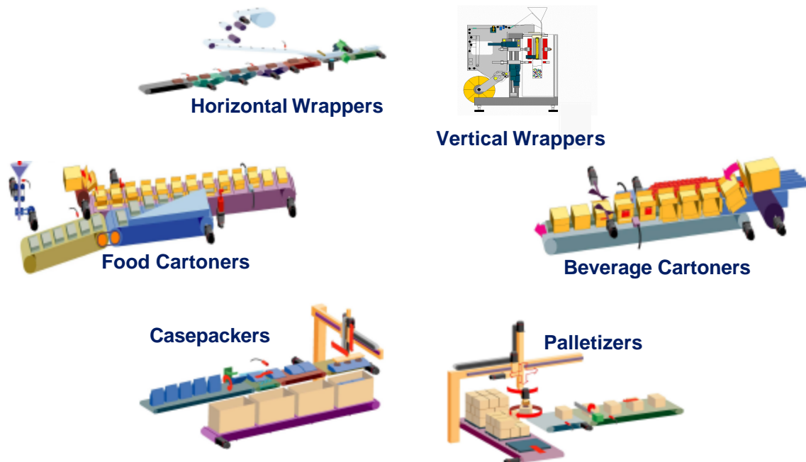
Figure 6: Distributed intelligence in packaging. Flow wrapper lines, vertical wrappers, case packers, food cartoners, smart belt systems, and thermoformers are some of the applications taking advantage of distributed intelligence in the servo drive.
