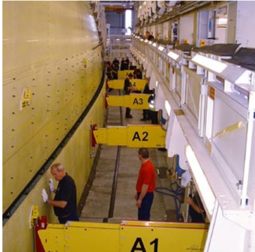
Closed-loop servo control provides fine position control with seamless transition between position and force control, as shown in this manipulation of a wing assembly for the Airbus 380.
