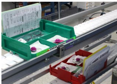
The system uses standard robotic trays barcoded with the patient’s prescription and frame style for automation processing.
