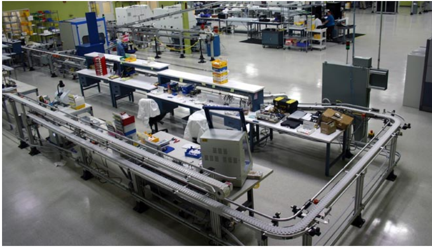
Ophthonix sends lenses to workstations using modular conveyors from Rexroth.
