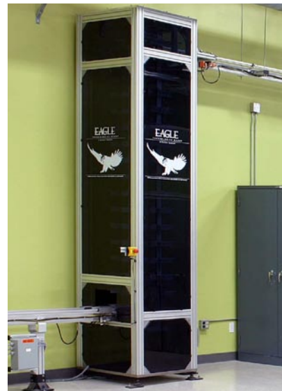
Using Rexroth aluminum structural framing, Eagle Technologies saved Ophthonix valuable floor space with this custom FIFO vertical buffer to transport trays to an overhead cooling line.
