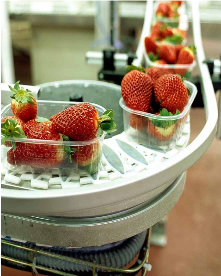
Curve wheels can reduce friction significantly in conveyors with 90° curves.
