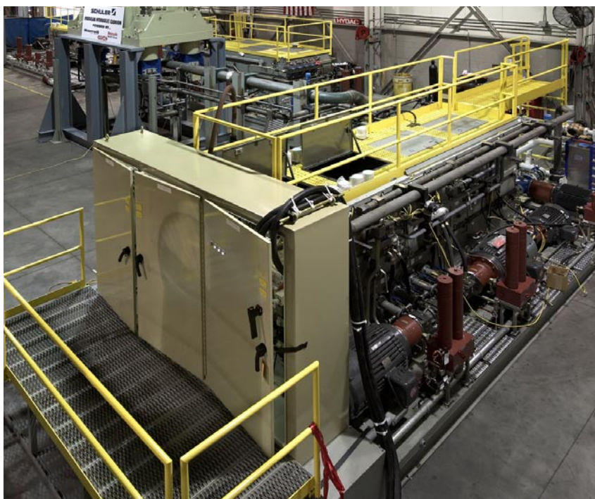
Hydraulic Power Unit for Schuler's Compact Crossbar Transfer Press
