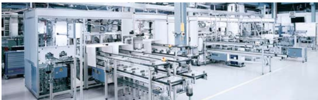
Customized assembly line, all over realised with the handling system camoLINE and transfer systems from Rexroth.
